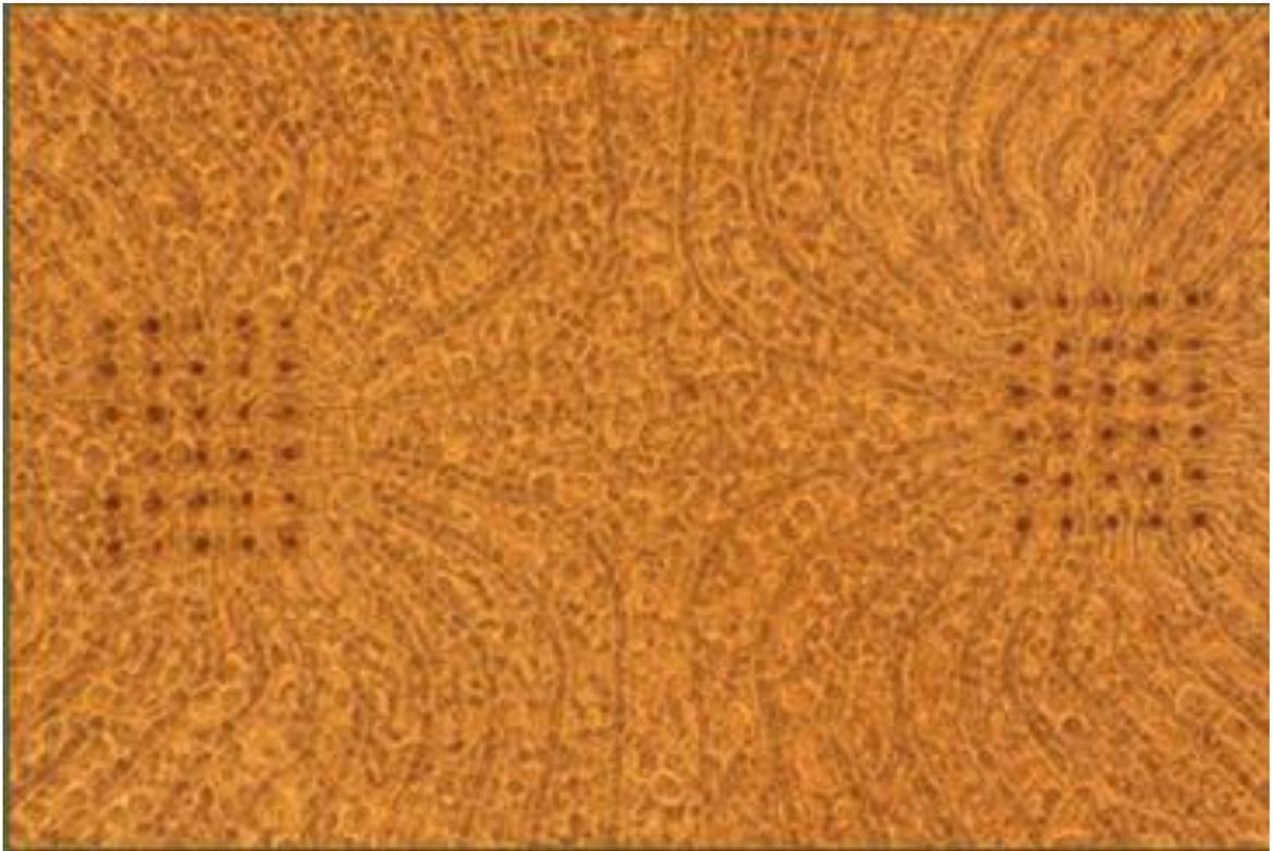
Figure 4.1. Phase contrast micrograph of the high-density electrode array, on which healthy neurons are growing. The HD array comprises two arrays of 6 X 5 electrodes (10  $\mu$ m diameter, 30  $\mu$ m spacing). The distance from center-to-center of the two electrode arrays is 200  $\mu$ m. The left half of the array was used in these experiments.
