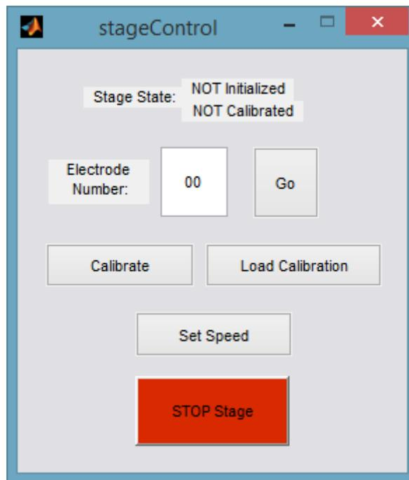
Figure A.1. GUI for controlling the automated stage movement.
