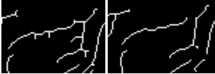
**Figure 53 – Skeleton fringe trimming, before and after.**
