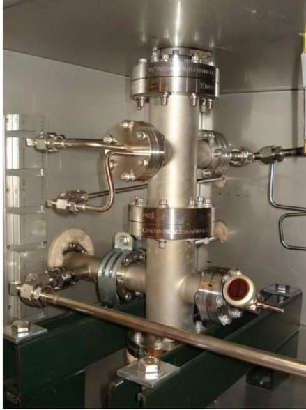
Figure 8: Picture of CVD deposition chamber.
