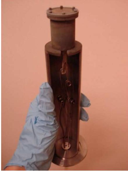
Figure 11: Picture of CVD heating assembly.
