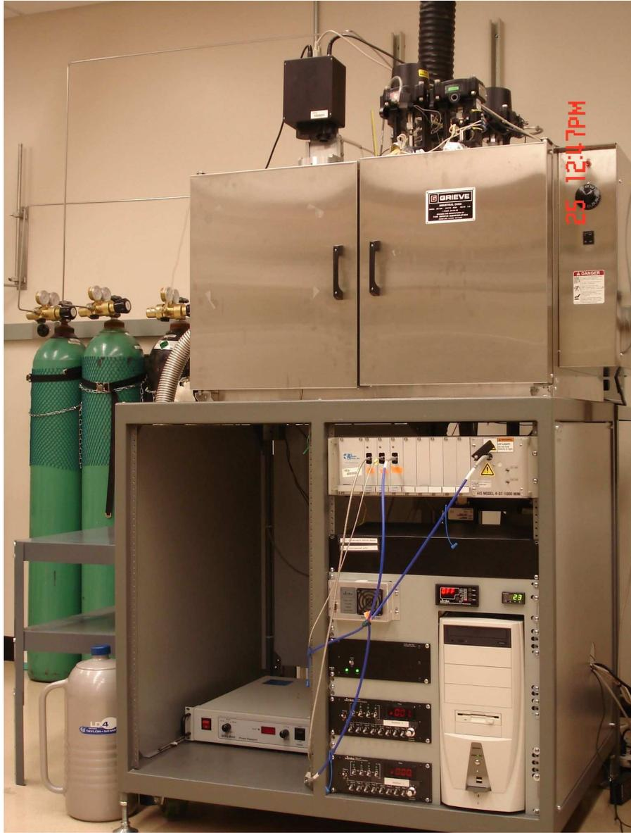
**Figure 2:** Photograph of the chemical vapor deposition testbed.
