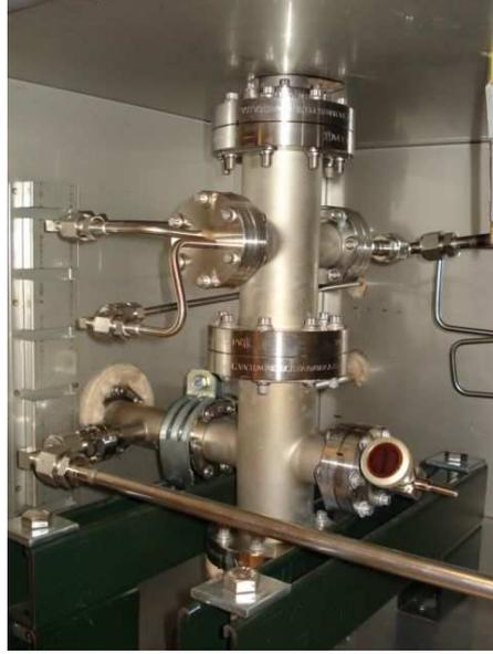
**Figure 3:** photograph of the chemical vapor deposition chamber.
