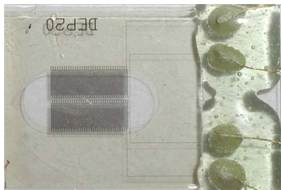
Figure 1. Completed electrode array with SU-8 layer to define measurement volume.
